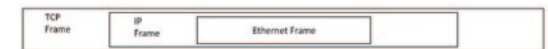
Continuing with our ‘box within-a-box’ or ‘envelope’ analogy, at the transport layer our IP frame is surrounded by a TCP frame, with is the predominant protocol in use at this layer.
