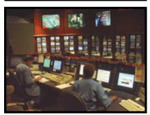
At this commercial insertion facility for a Cox cable headend in San Diego, operations mainly center on ensuring that commercial media and other interstitial material is available and that playlists are complete and correct. The video switcher seen on the console is used only during live sporting events. In all other instances, program stream switching and other transitioning is handled under automation control.
