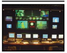
As program services and requirements change, this rear-projection "glass cockpit" monitor wall can recall multiple configurations of source monitoring.
