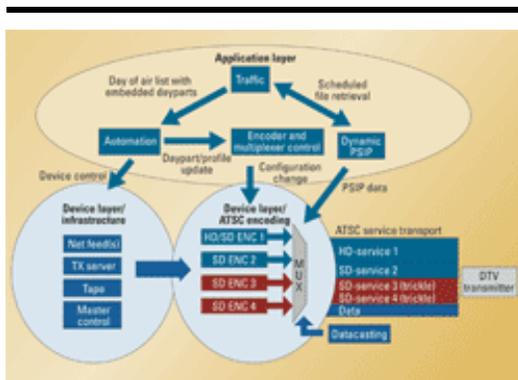
Figure 4. In multichannel broadcasting, a large part of the master control operator's job is reacting to system faults, and keeping program logs up-to-date across channels. [Click here to see an enlarged diagram.](#)
