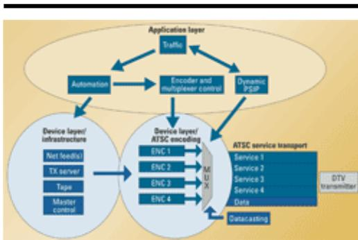
Figure 1. In multichannel operations, the application layer gets larger and more processes must collaborate to effectively manage the additional services. Click [here](#) to see an enlarged diagram.
